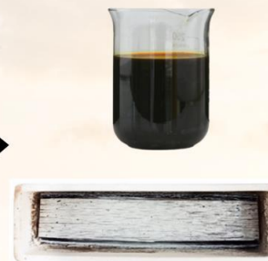
Fig. 15. Pyrolysis oil and raw materials of wind turbine blades after pyrolysis 15, 13 .
