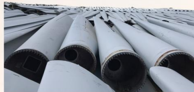
Fig. 14. Wind turbine blade waste 14 .
